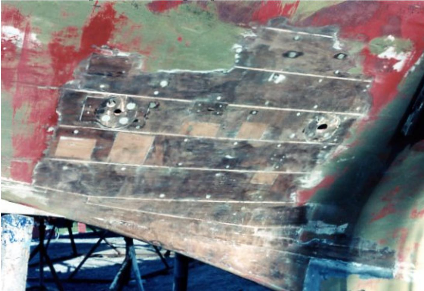
Despite Lloyds classification surveys every two years from new, many small bits of poor workmanship had crept in since 1961 and the first few years of my ownership were spent in upgrading and replacing some of the mahogany planks. These “graving pieces” had been fitted over the top of plank fastenings, concealing soft areas. Final solution; replace the planks....
