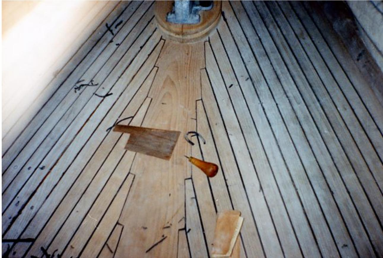
Due to over-scrubbing in the past, the deck required regular attention. However we managed to keep it watertight up to 1997 and I believe it has only required rebuilding in the last year or so – see 2009 pics below....
