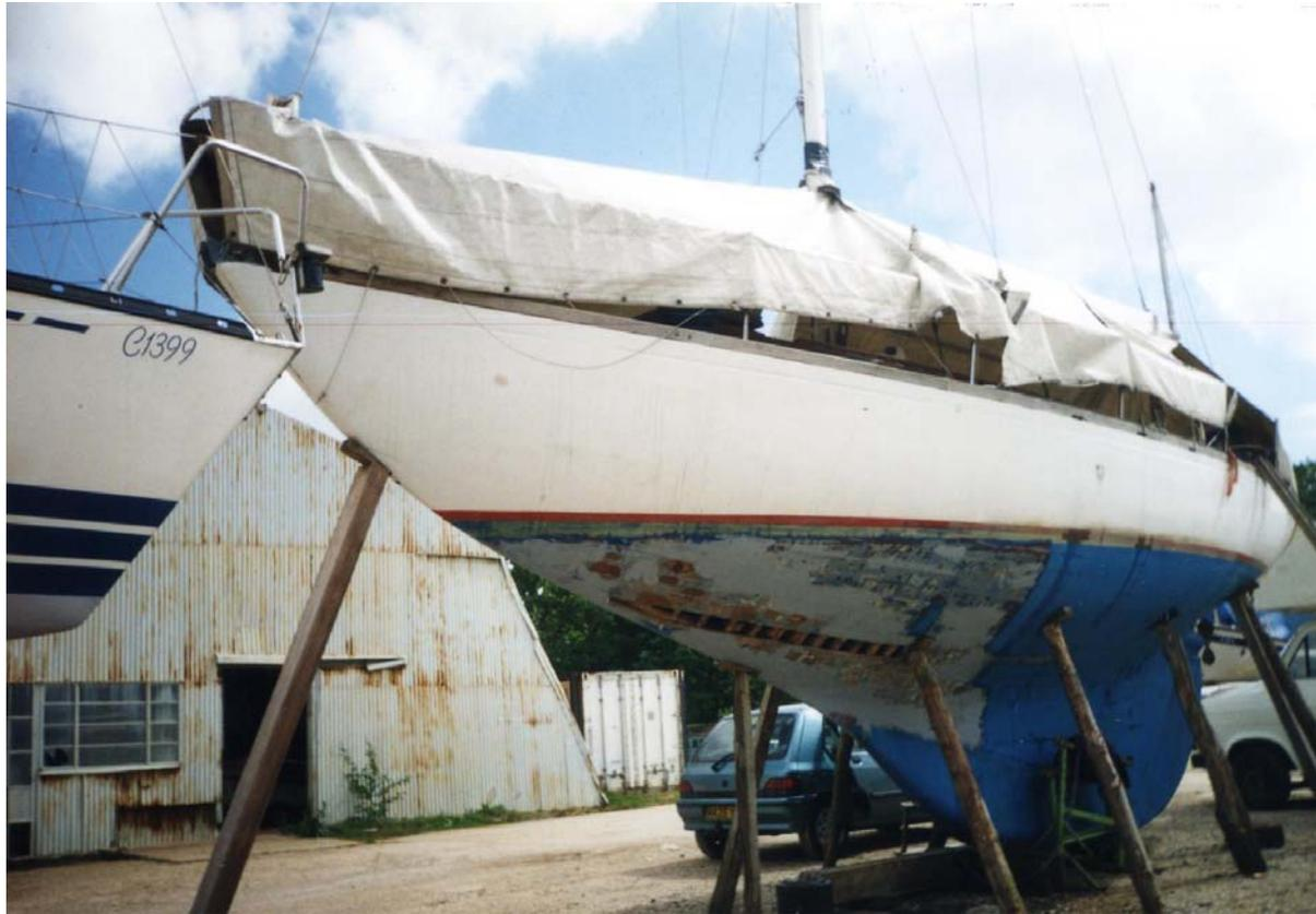
An overall cover for a timber boat is an absolute essential. Even trakmark decks on a modern GRP hull benefit from being covered - it saves a lot of scrubbing.
