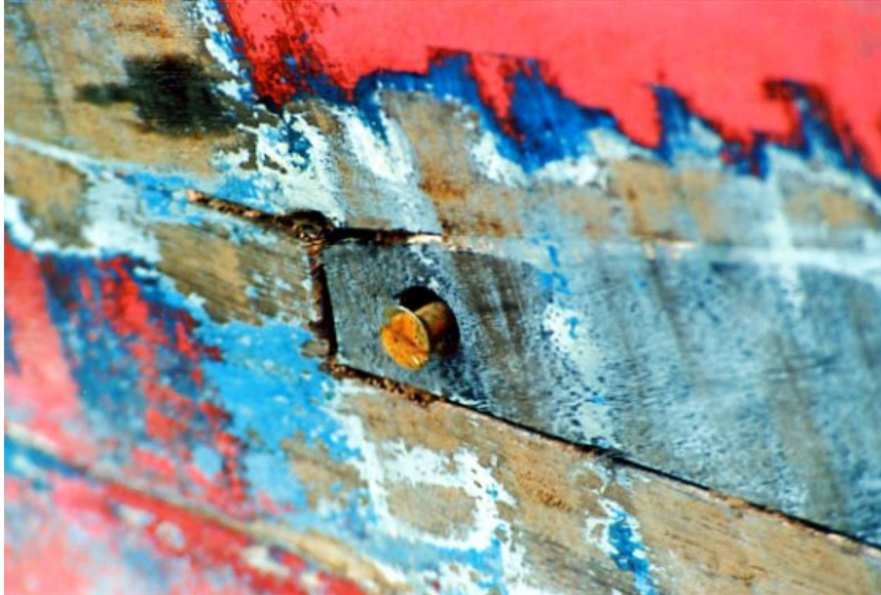
For every Lloyds inspection, at 2-year intervals, plank fastenings, keel bolts, rudder stock, chain-plate bolts etc had to be removed in rotation. Had I not sold the yacht, I would have removed her from Lloyds class as the cost of the surveys plus the work involved became prohibitive and the destructive effect on the boat very noticeable.
