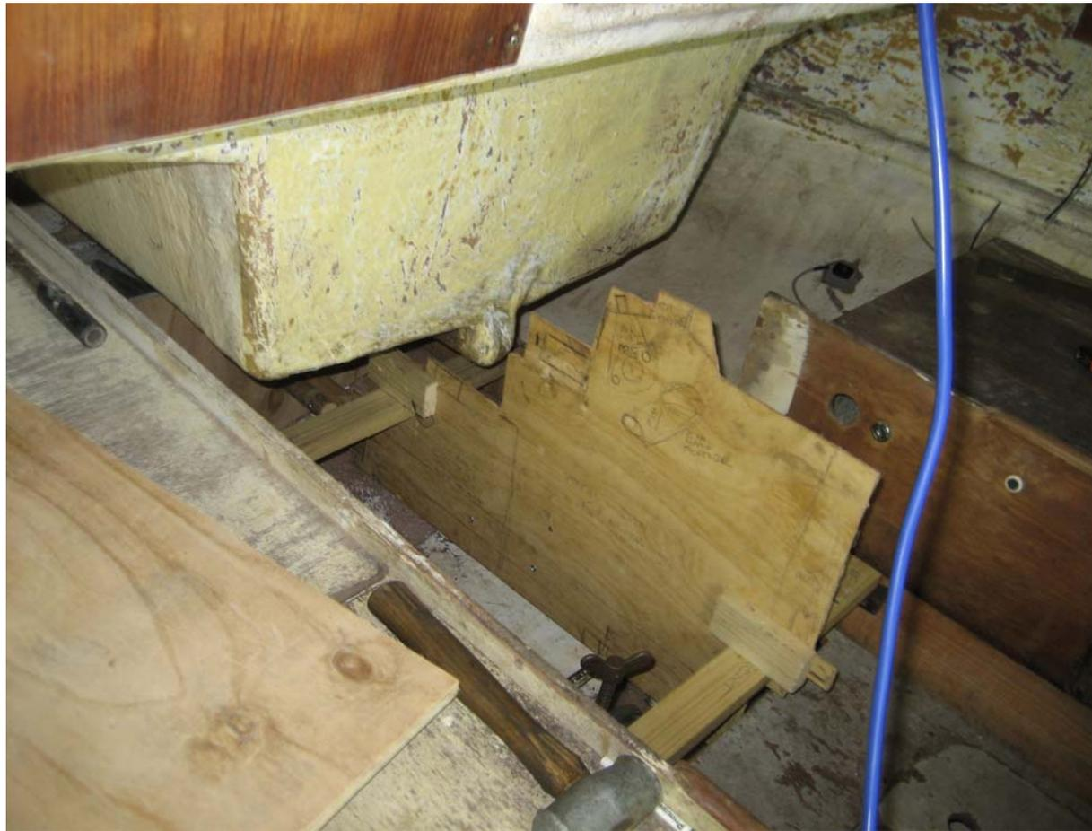
Using the maximum deflection of the Aqua-drive joint, the engine can be installed horizontally, which only means 4" extra on the engine box height.
