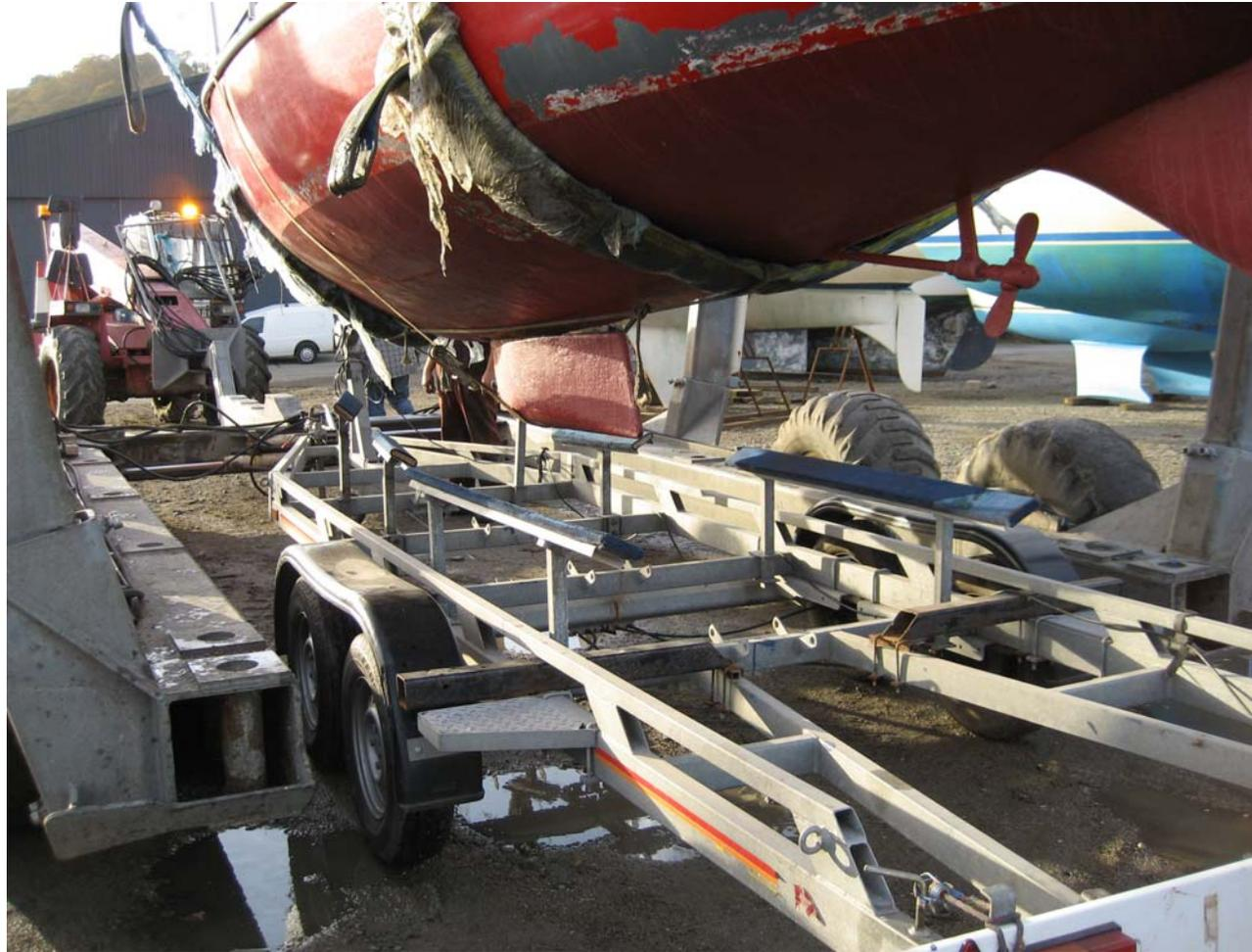
The trailer was actually designed for a bilge-keeler, so a bit of hocus-pocus was necessary to get the boat to fit.....
