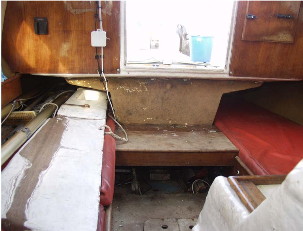
The original Watamota Sea-Nymph crawled out and died some years back. The current outboard-engine arrangement is being replaced by a reconditioned 1972 Lister Petter 1ACW inboard Diesel (70Kg), the same age as the boat.
