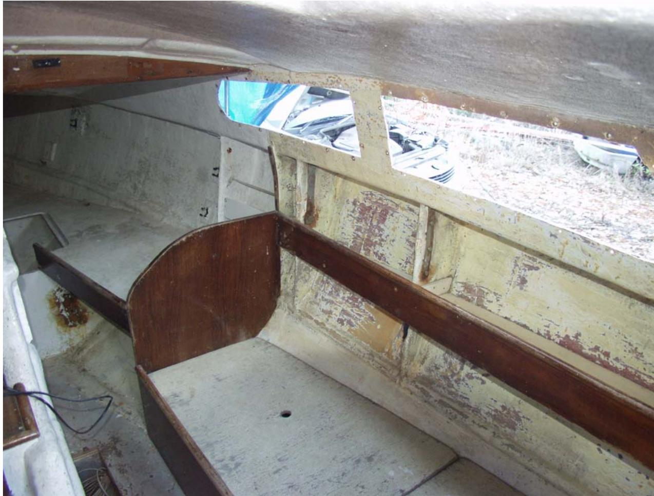
The worst bit to prepare was definitely the cabin roof, which had been painted with some weird gloop. I tried chemical stripper, blowlamp etc etc and ended up using good old-fashioned elbow-grease and a scraper.
