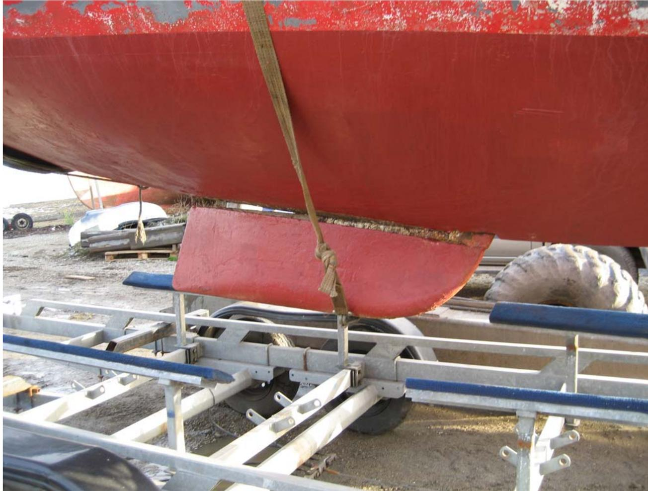
A half-ton of cast iron looking for a way down.....
