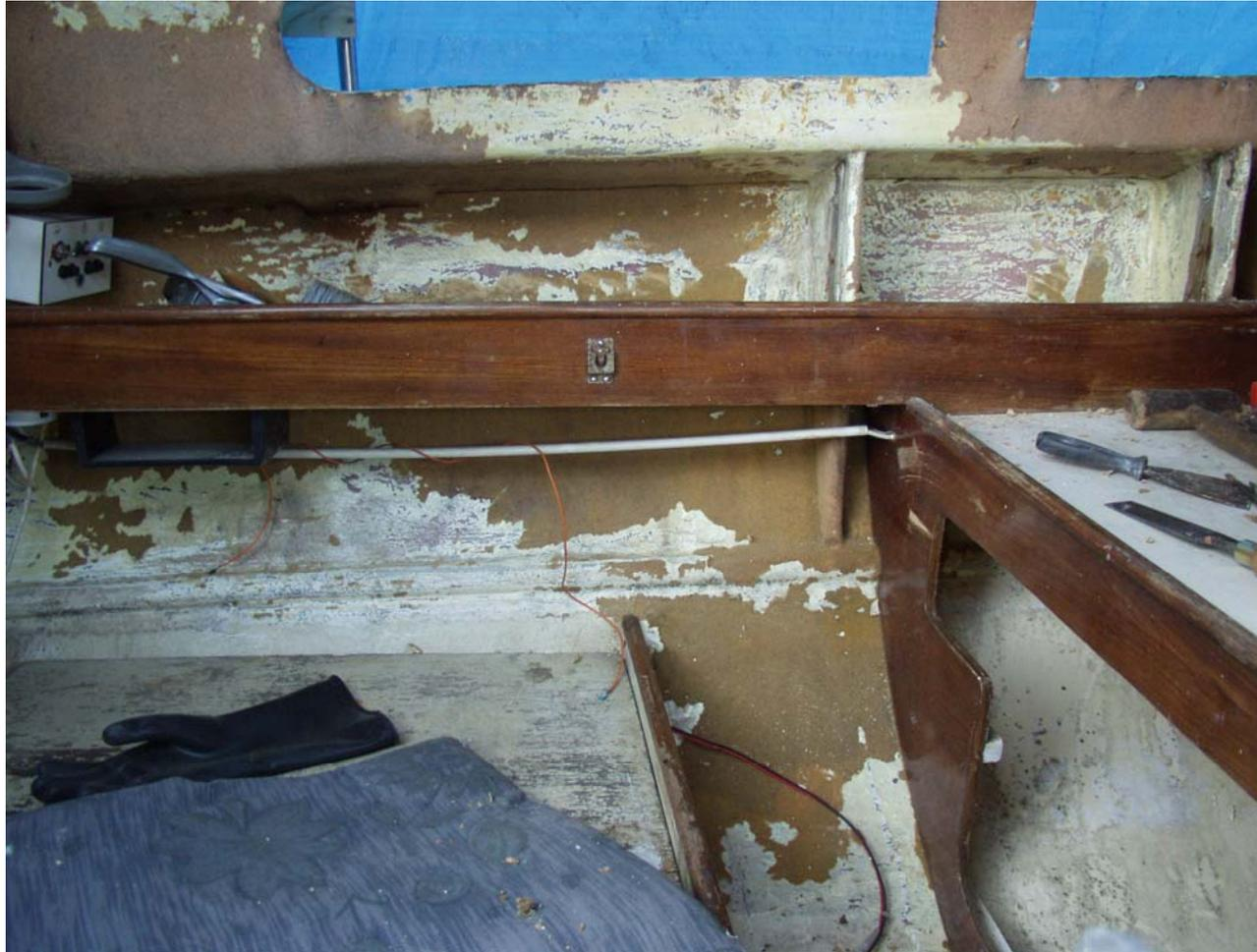
Every square inch of the inside has been stripped using a hand scraper. The coating seen here was a typical 1970's "furry" sprayed-on material. Very difficult to shift, as chemicals had no effect whatsoever ...
