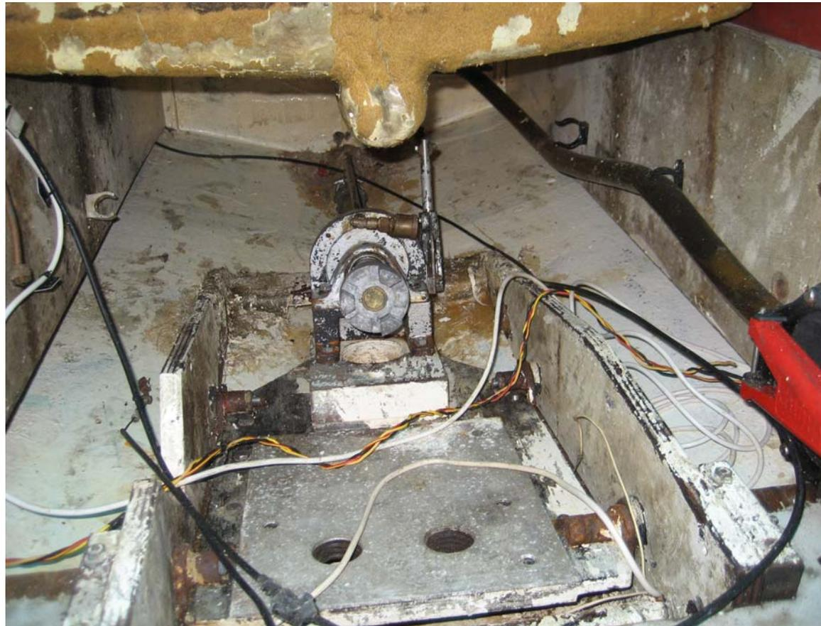
A very clever little piece of engineering, but the propeller gears were corroded and spares not available - or I would have used the system with the replacement Lister-Petter diesel engine, to save 25kg of weight.
