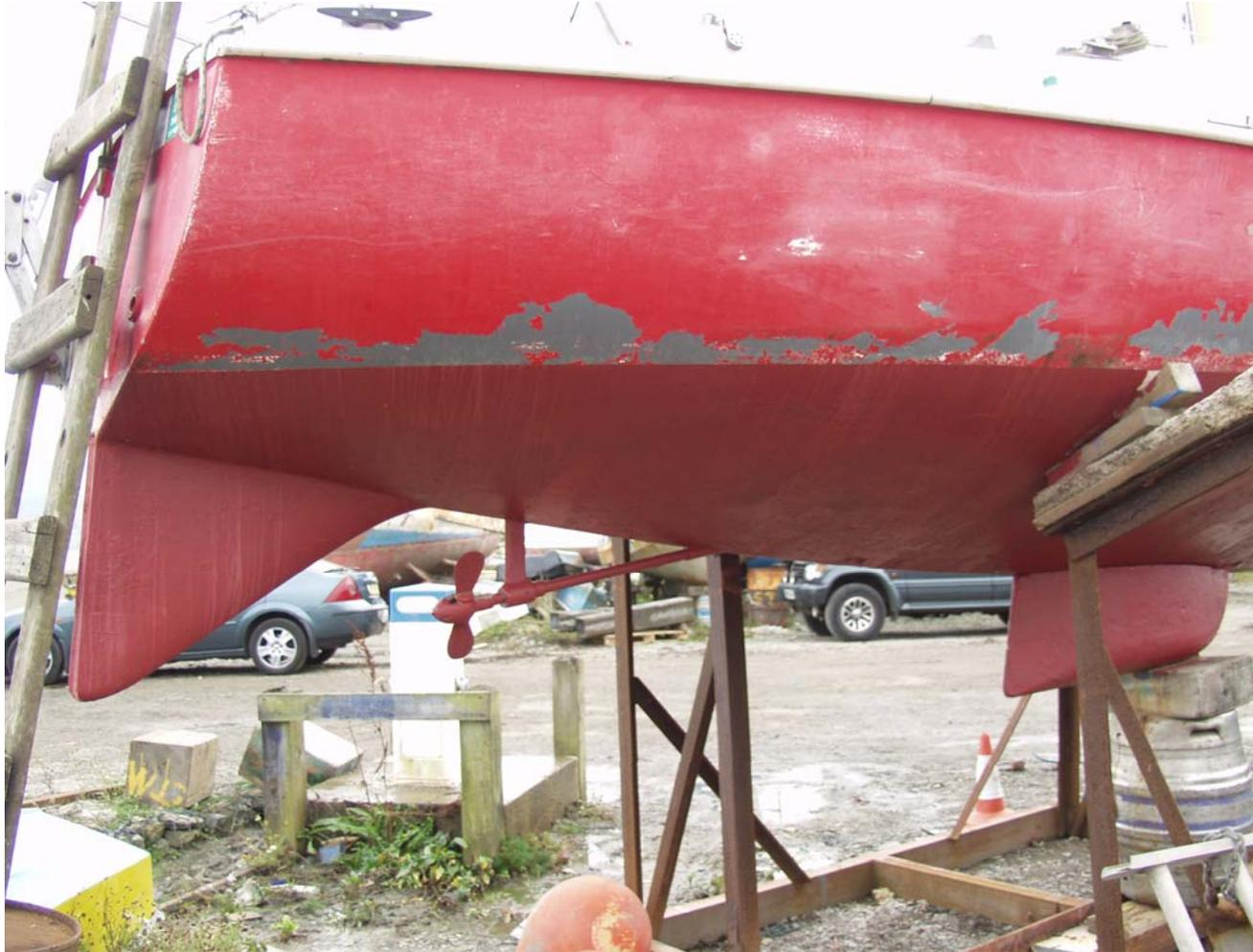
.....all of which had left large areas of exposed laminate. The results of this vandalism had been concealed by a freshly applied coating of anti-fouling.
