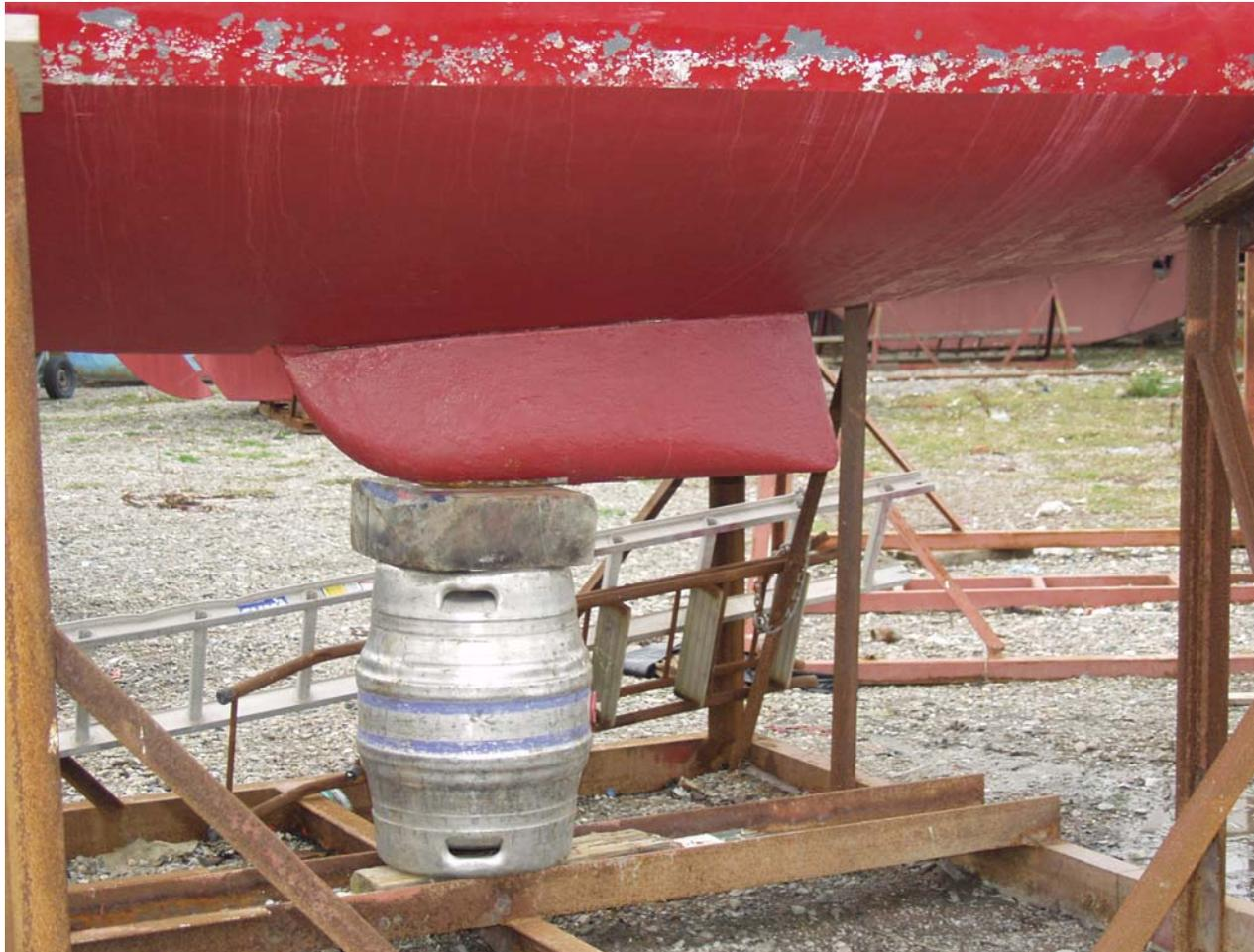
The hydraulics had been disconnected, which would have allowed the keel to free-fall if left unsupported. This would act like a half ton hammer on the GRP keel-box.....
