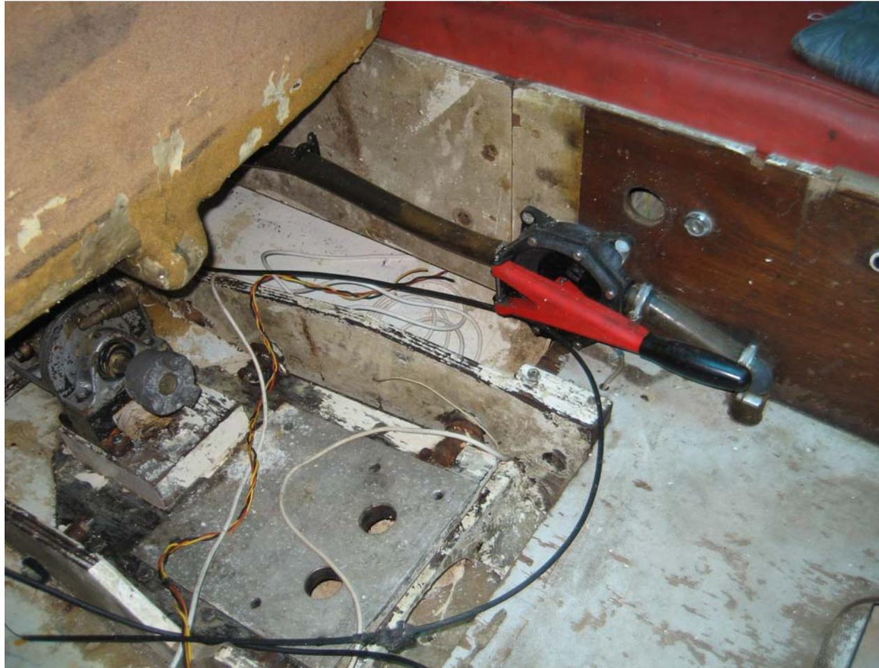
An “Aquadrive” constant velocity coupling and folding propeller are being installed, together with double acoustic-silencing foam to the engine box. This will result in a quiet and smooth engine, hopefully.
